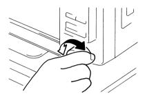
When the Image Rotation Knob is turned while holding down the Shift Key, the image quickly rotates by 90°.
